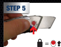
STEP 5 Once blade has retracted, flick red button to 'lock' position
