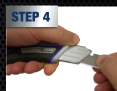
STEP 4 While holding the blade slider, pull out the blade and replace with new one
